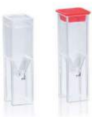
Method: The graph and the table display the precise light transmission of the cuvette depending on the different wavelengths and the different plastic types. Cuvettes each filled with distilled, clear water. Optical path length 10mm
